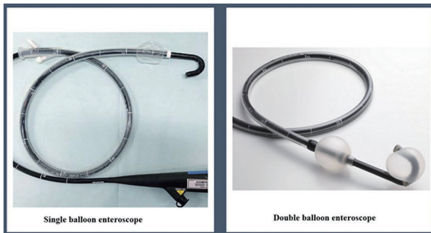
Fig. 1. Short-type single and double balloon enteroscopes (courtesy of Olympus, Tokyo, Japan; FUJIFILM, Tokyo, Japan).
